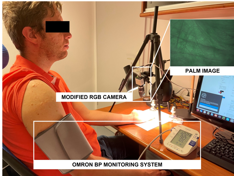
Figure 5.2: Anonymous subject being recorded with our custom camera and BP recording setup. Picture used with subject's explicit permission.
