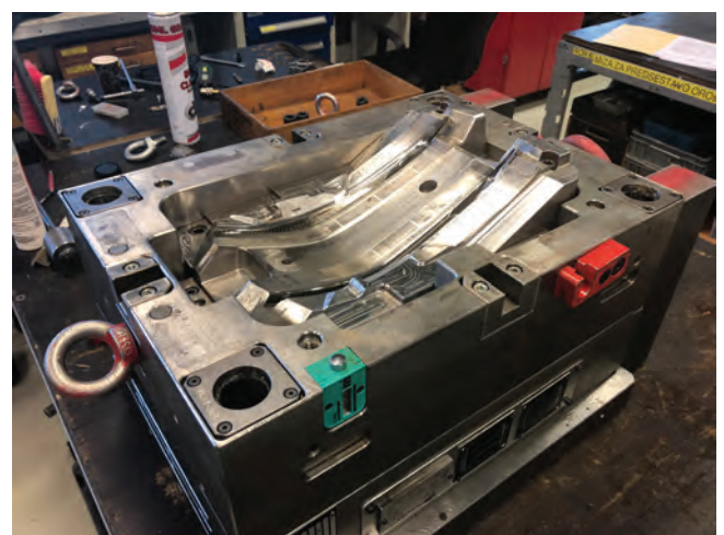
Figure 1: To improve the planning of tool manufacturing for injection molding, we developed a software solution to predict the duration of machining operations that relies on extracting features from 3D tool drawings and machine learning of predictions based on these features.
