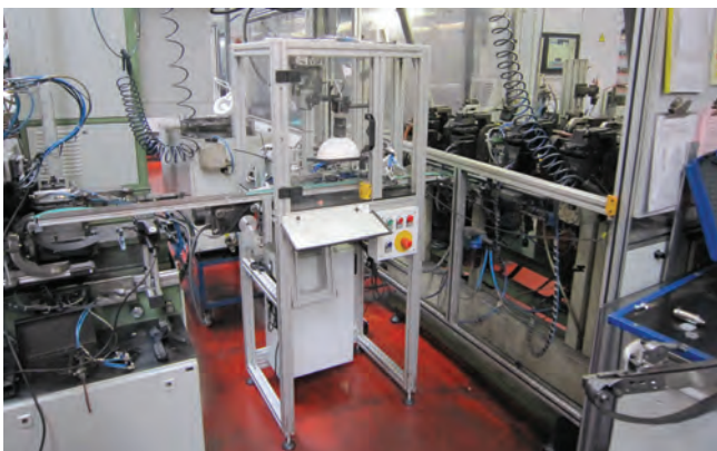
Figure 3: A manufacturing quality control system resulting from the COPCAMS project is based on machine vision, machine learning and optimization.
