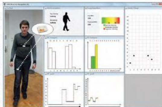
Figure 1: Human activity recognition and energy expenditure estimation with accelerometers in the Chiron project
