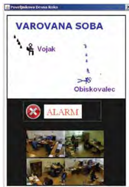
Figure 1: The control panel of the intelligent security system ("PDR" project), where the situation in the surveilled rooms is presented with a live picture, a symbolic-graphical and textual description.
