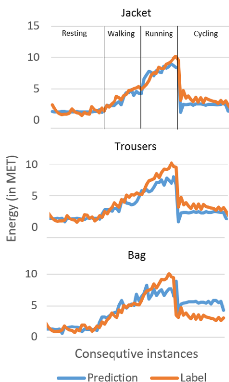
Fig. 7. Comparison of the estimated and ground-truth energy expenditure. The labels on top indicate in the location of the phone and the activity.
