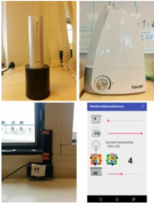
Figure 3: Devices used in the experiment. Indoor NetAtmo™ module (top left), humidifier (top right), window state sensor (bottom left), and application interface for self-reporting the occupancy, labeling the state of the used devices and receiving the recommendations (bottom right).
