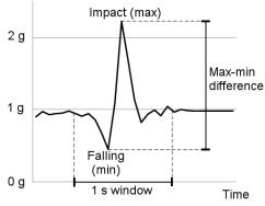
Figure 1: Acceleration pattern during a fall.
