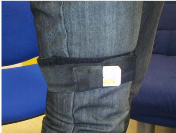
Figure 1. Shimmer inertial sensor attached to the thigh.
