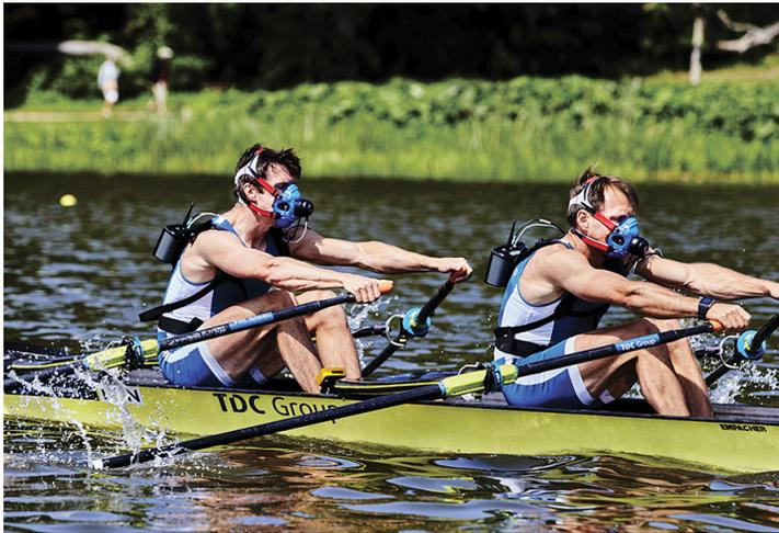
Fig. 3. Cosmed K5 portable indirect calorimeter from <http://www.cosmed.com/en/products/cardio-pulmonary-exercise-testing/k5>.
