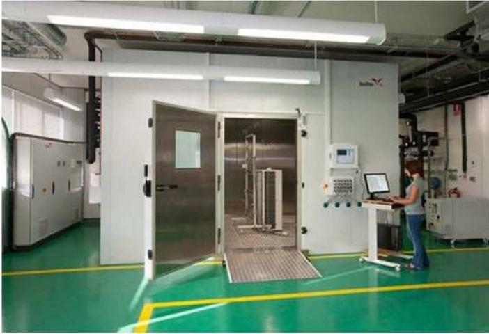
Fig. 2. Direct calorimeter chamber from <http://www.directindustry.com/prod/ineltec-france/product-123381-1399577.html>
