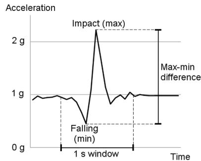
**Fig. 4.** Acceleration pattern during a fall
